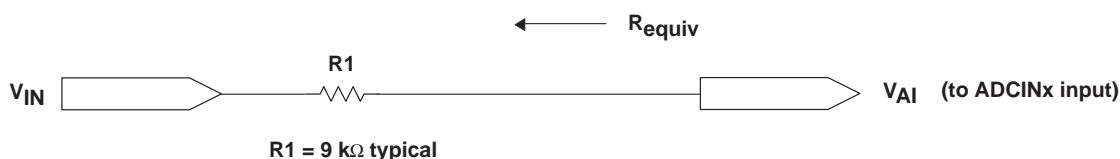
Figure 47. Typical ADC Input Pin Circuit
